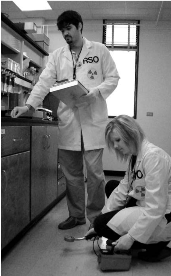
Above: RSO staff perform leak test analysis for the sealed radioactive source using an alpha-beta proportional counter.
